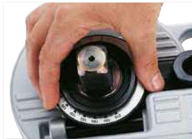
Manual adjustment of the bending angle from 0° to 180°.
